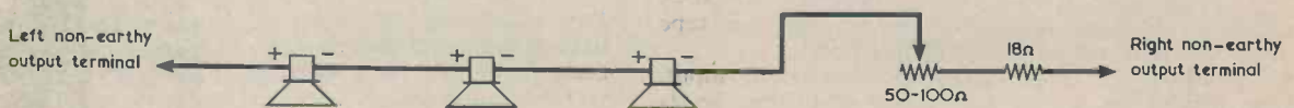
Fig. 8. One or more speakers at the back can increase the apparent spatial effect of the sound source
